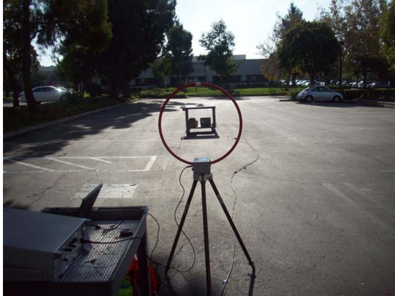
RADIATED EMISSIONS BELOW 30MHz (FRONT)
