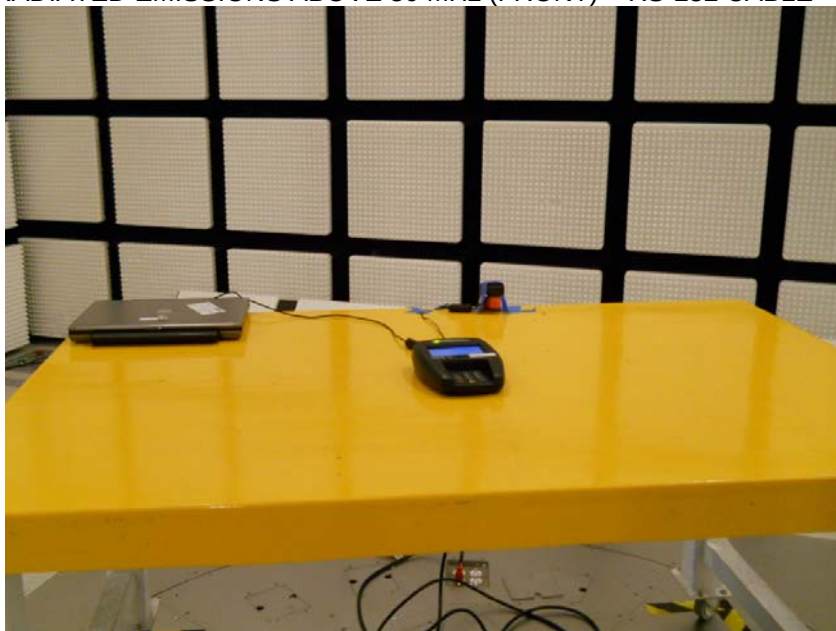
RADIATED EMISSIONS ABOVE 30 MHz (FRONT) – RS-232 CABLE
