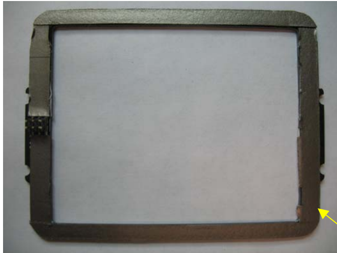
IMG_0663 Antenna Board [bottom view of antenna board with ferrite]
