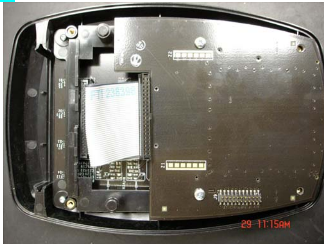
SC07233 (EUT when opened top portion)
