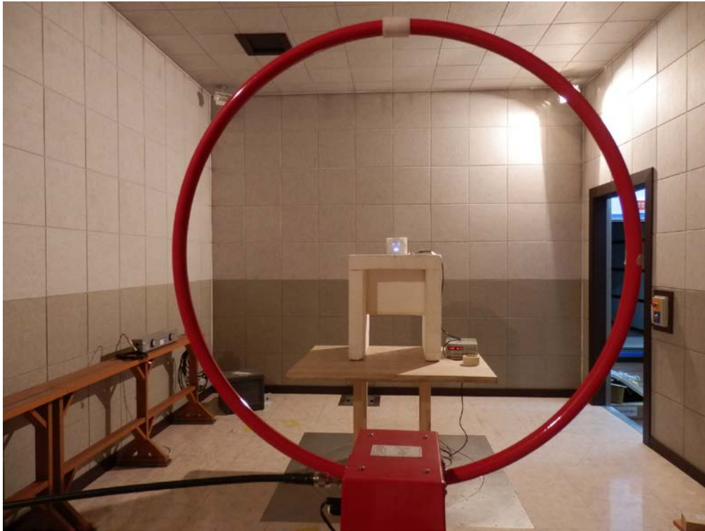
Photograph 1: Test Setup for 9 kHz to 30 MHz
