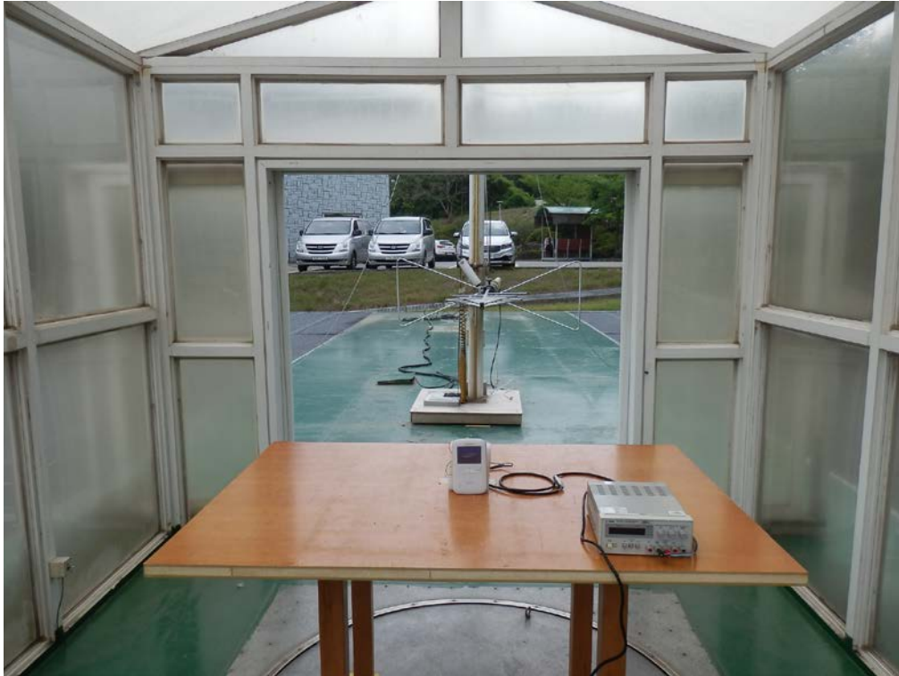
Photograph 2: Test Setup for Below 1 GHz
