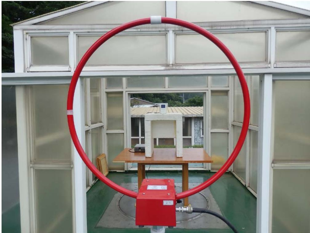
Photograph 1: Test Setup for 9 kHz to 30 MHz
