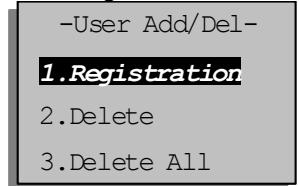
3. When the LCD screen displays “Approach card to be registered”, place a user access card over the card reader.
