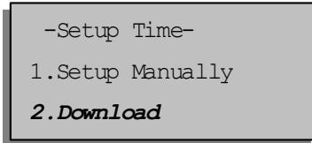
This function enables the reader to be synchronized with the Attendance program (server) time. In this case the reader needs to be connected to the server.
