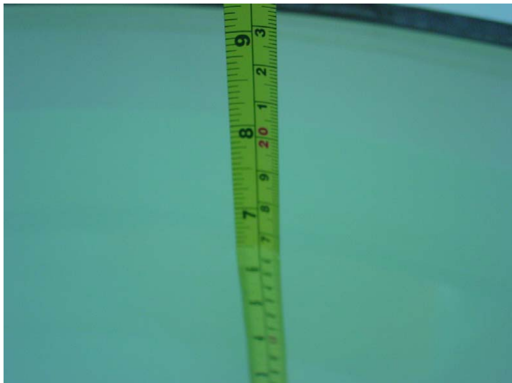
Picture B2: Liquid depth in the Flat Phantom (450MHz Head)
