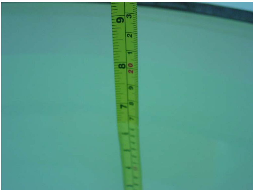
Picture B3: Liquid depth in the Flat Phantom (450MHz Body)
