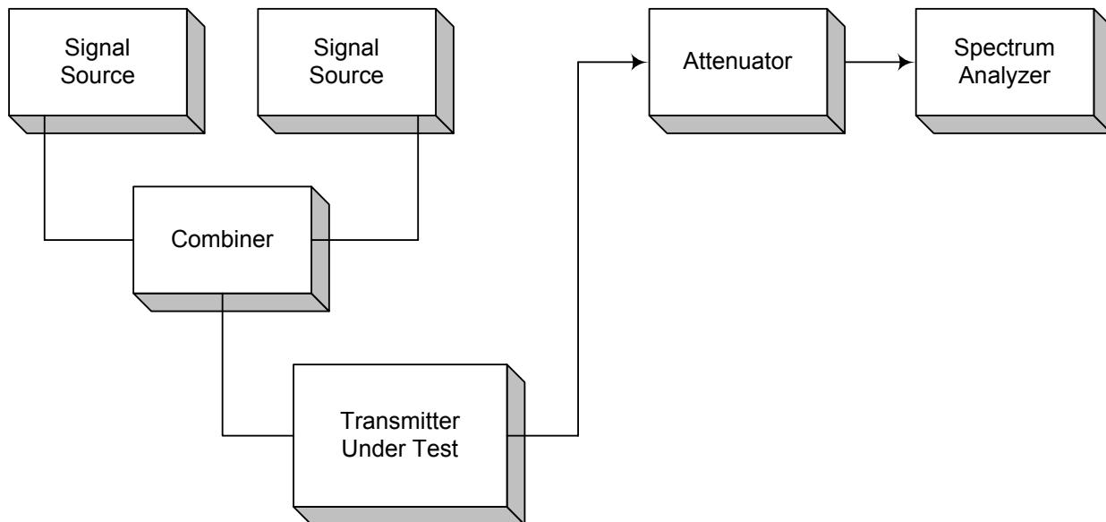
**Para. No. 2.991 - Spurious Emissions at Antenna Terminals**
