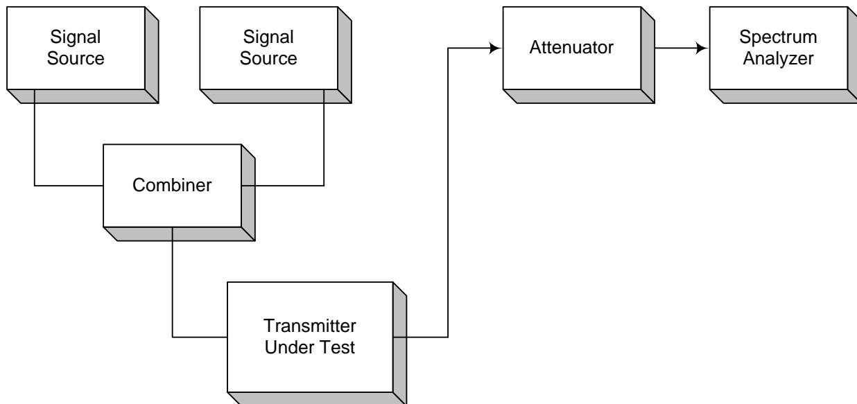
**Para. No. 2.991 - Spurious Emissions at Antenna Terminals**
