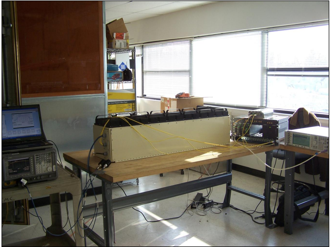
Photograph 5. Conducted Spurious Emissions, Test Setup
