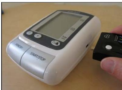
1. Plug Ambio Wireless Connector into the meter (if not already attached).
