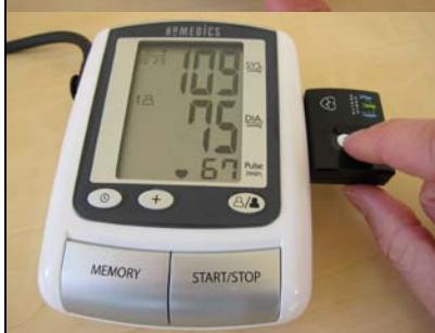
4. Readings are automatically sent to the Ambio Care Portal up to three times per day. Press the button on the Wireless Connector if you want to send the reading immediately. If you are not within range of the Gateway, readings will be stored in the meter and transmitted when you are back in range.
