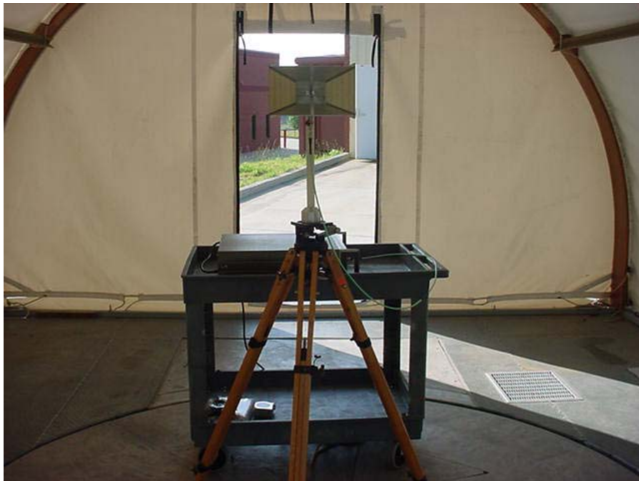
Figure 3: Substitution Field Strength – Front View
