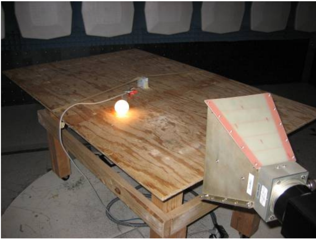
Radiated Emission Setup View (> 1GHz)
