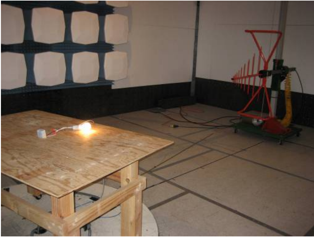
Radiated Emission Setup View ( < 1\text{GHz} )
