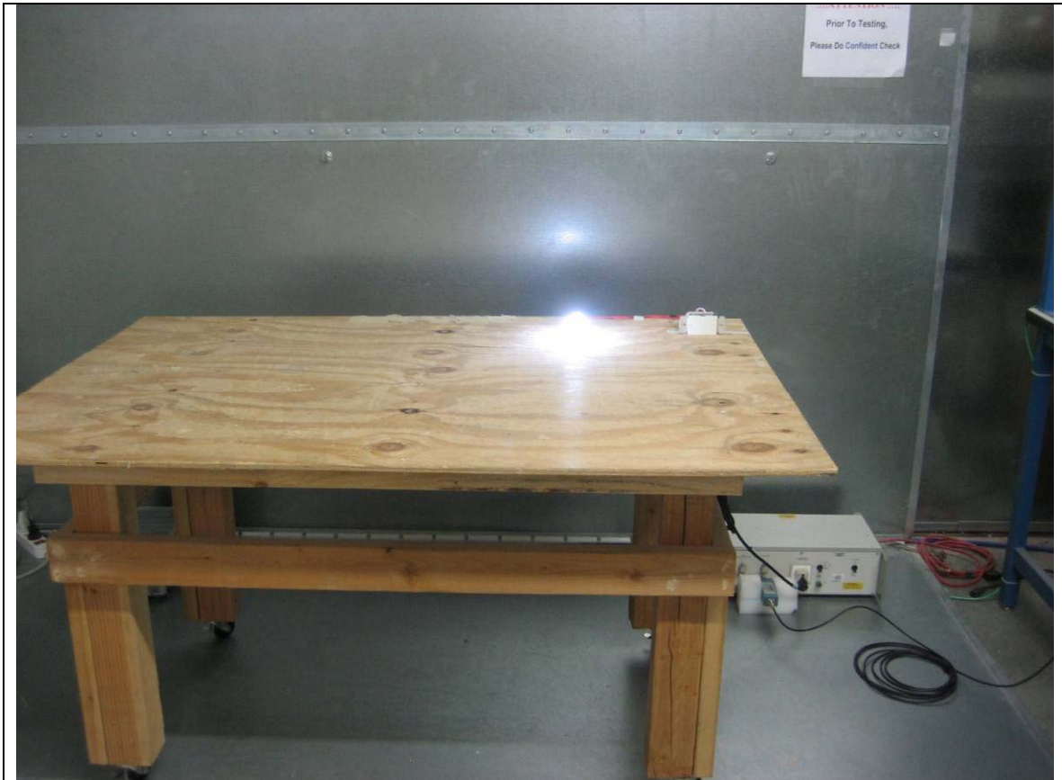
Conducted Emission Test Setup – Front View
