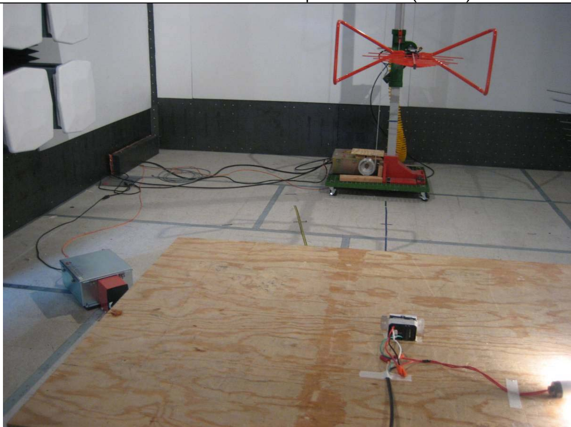
Radiated Emission Test Setup – Rear View (<1GHz)
