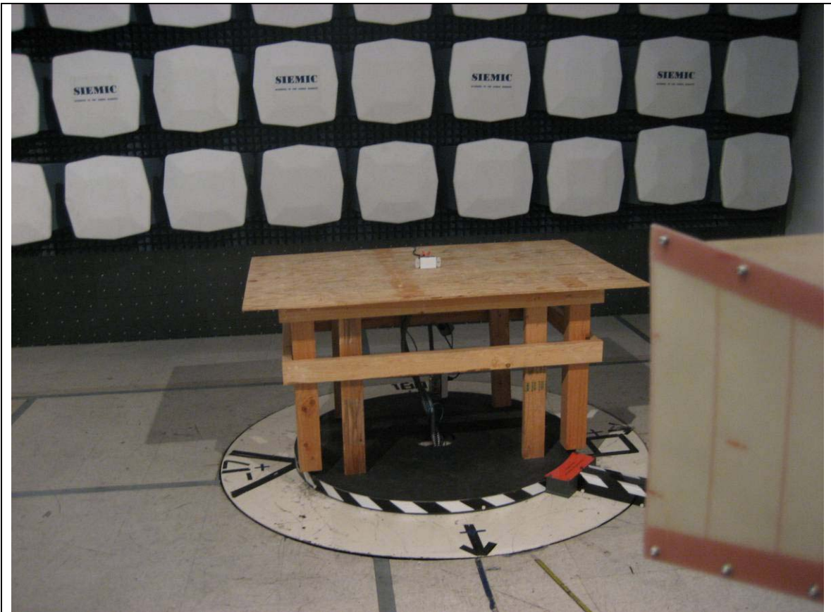
Radiated Emission Test Setup – Front View (>1GHz)
