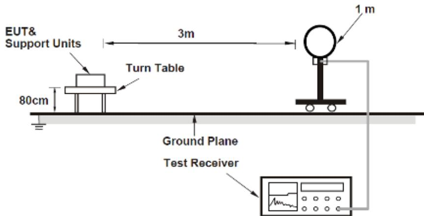
For Radiated emission 30MHz to 1GHz
