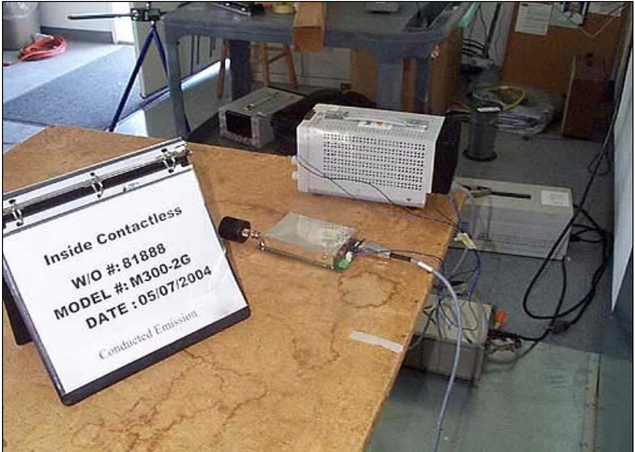
Mains Conducted Emissions - Back View
