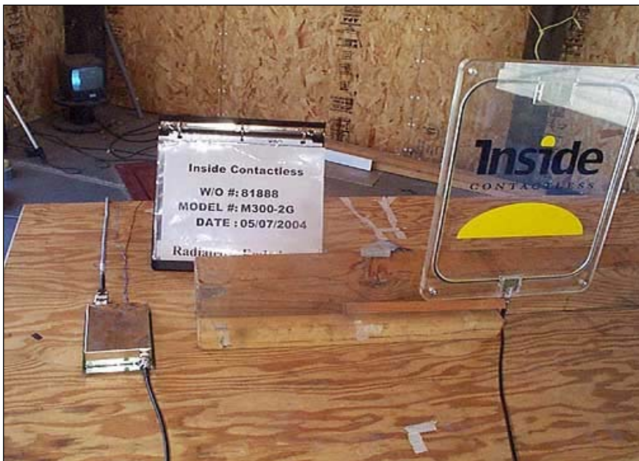
Radiated Emissions – Back View
