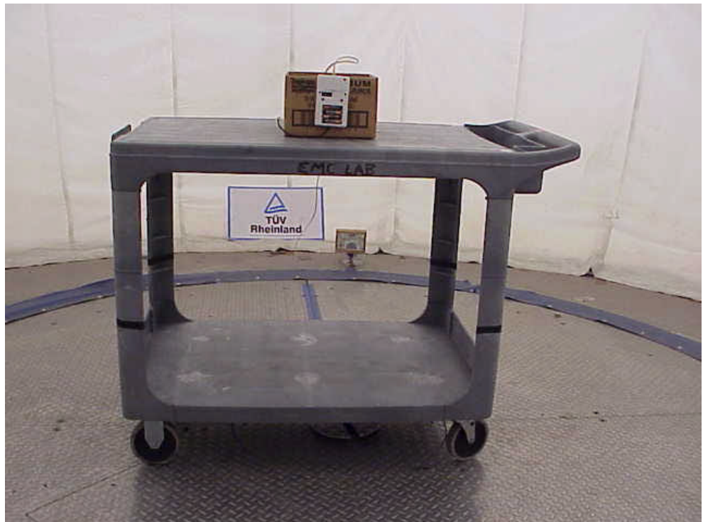
Radiated Emissions test setup in OATS
