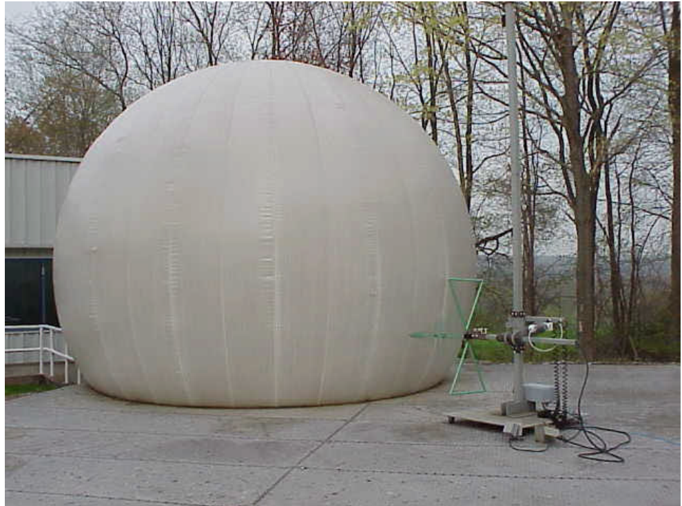
External View of Radiated Emissions test setup in OATS Antenna shown in 3m position
