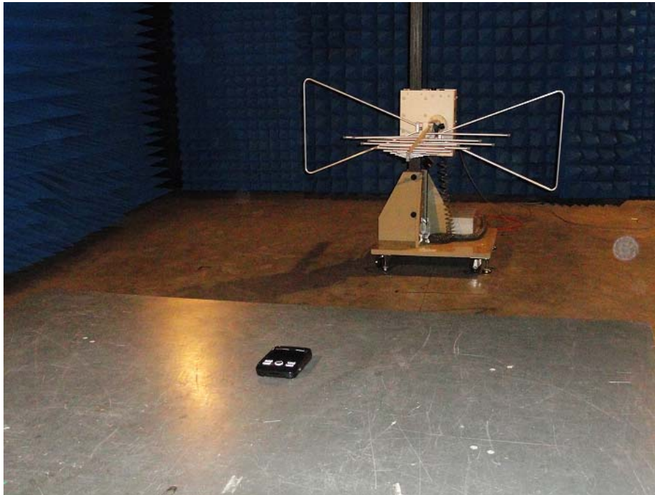
Radiated emission test view
