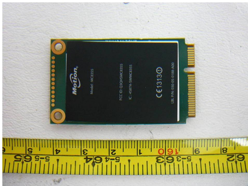
**12.13 EUT –WLAN/BT Combo Module Top View without Shielding**
