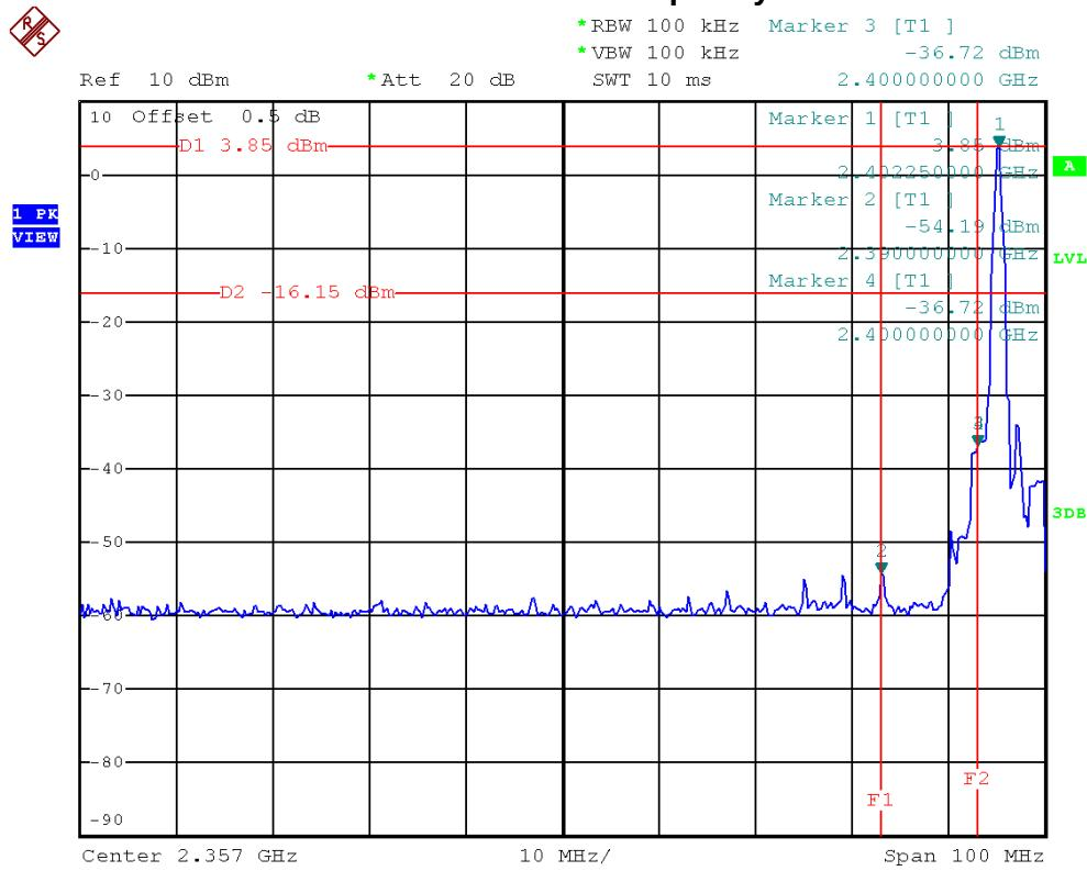
**Bluetooth / 1 Mbps / CH78-The max. radio frequency power in any 100 kHz bandwidth within the frequency band**
