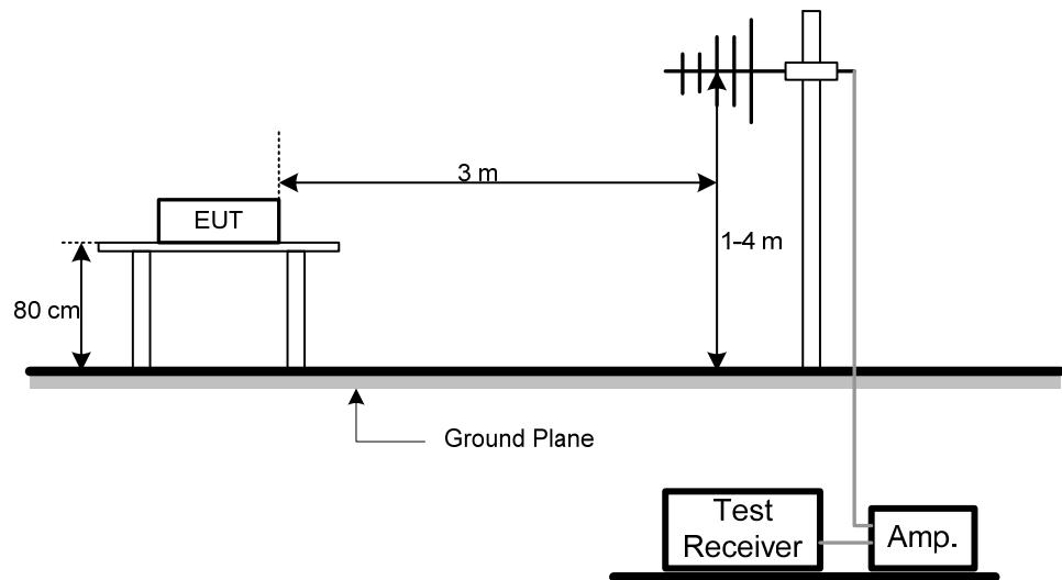
**Radiated Emission Test Set-Up Frequency Above 1 GHz**
