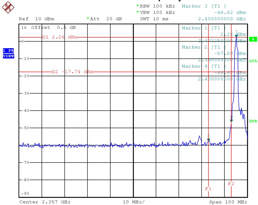
**Bluetooth / 3 Mbps / CH78-The max. radio frequency power in any 100 kHz bandwidth within the frequency band**
