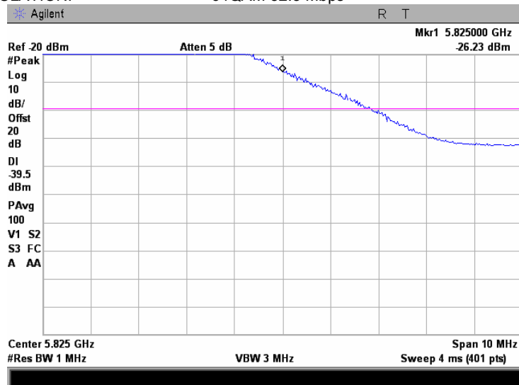
Plot 7.5.59 Conducted spurious emission measurements at the band edges
