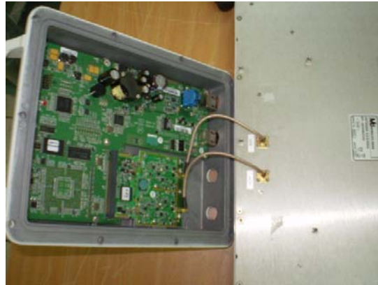
Photograph 7.7.2 Antenna assembly, integrated
