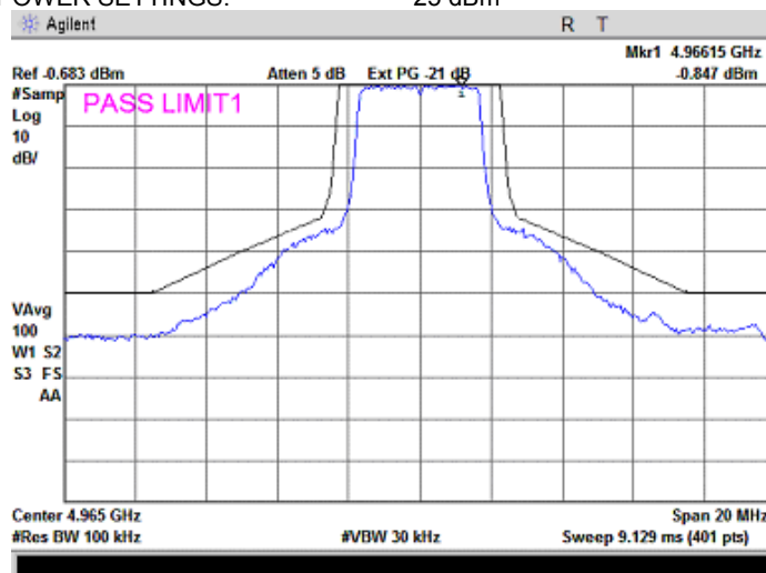
Plot 7.3.6 Emission mask test results at high carrier frequency
