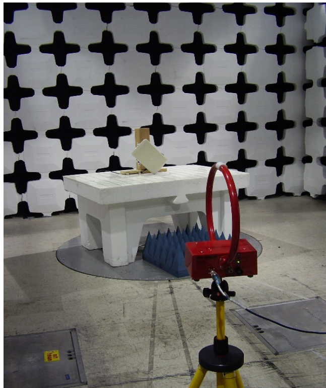
Photo 4. Radiated emission test setup with Loop antenna.
