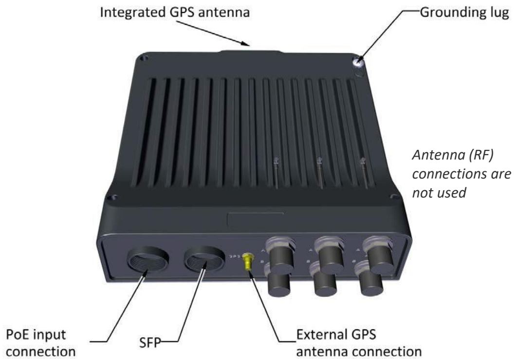
Figure 2-54: OSU external connections
