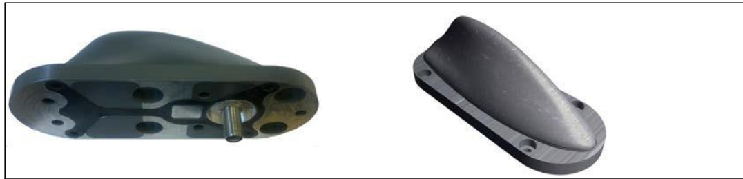
Figure 2-87: "Shark-Fin" antenna - bottom and top views
