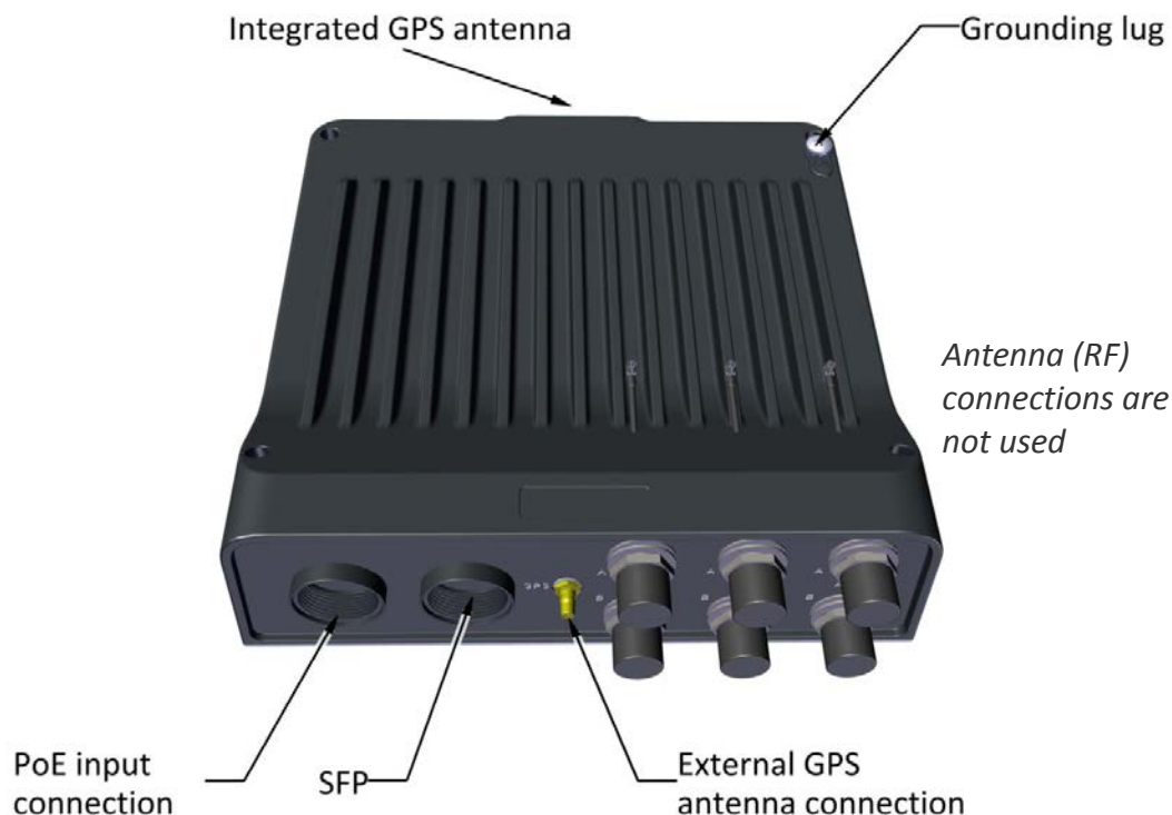
Figure 2-54: OSU external connections
