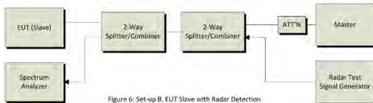
A full system calibration was performed on the test station and any resulting system losses (or gains) were taken into account in the production of all final measurement data.
