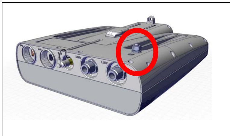
Figure 2-22: Ground: HBS radio unit
