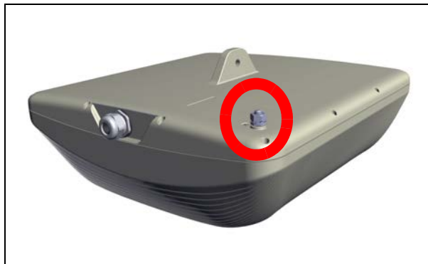
Figure 2-23: Ground: SU radio unit
