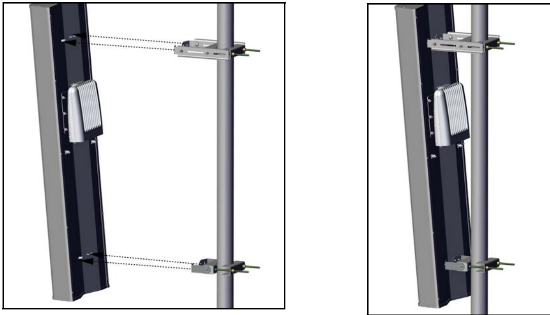
Figure 2-6: Mount HBS/ antenna on pole
