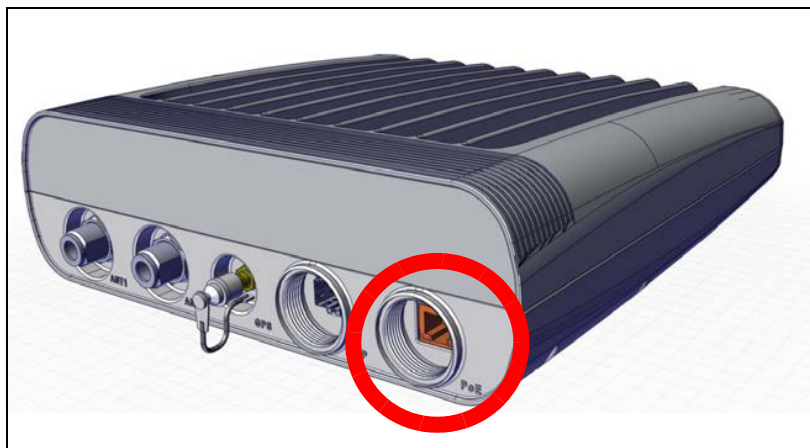
Figure 2-26: Input port: HBS unit (connection label: "PoE")
