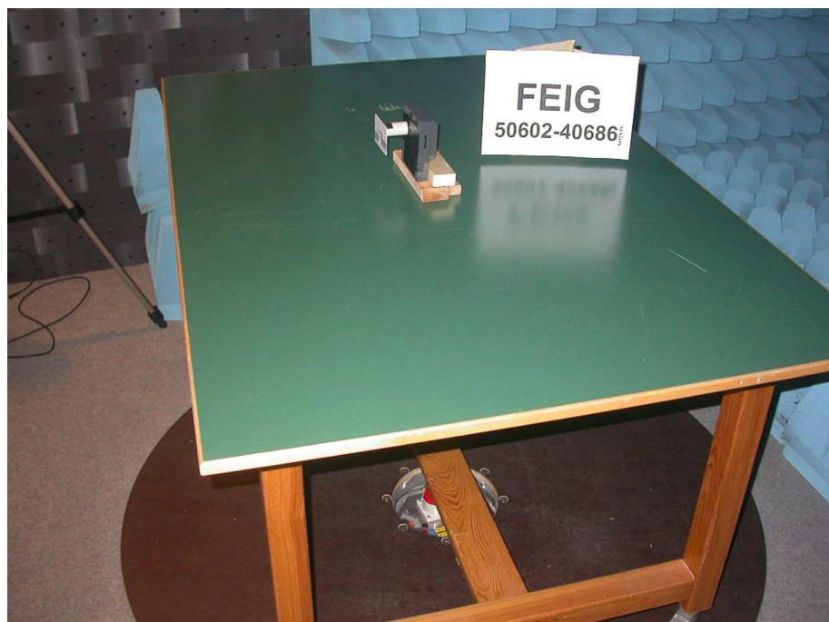
**Test setup for radiated emission test
