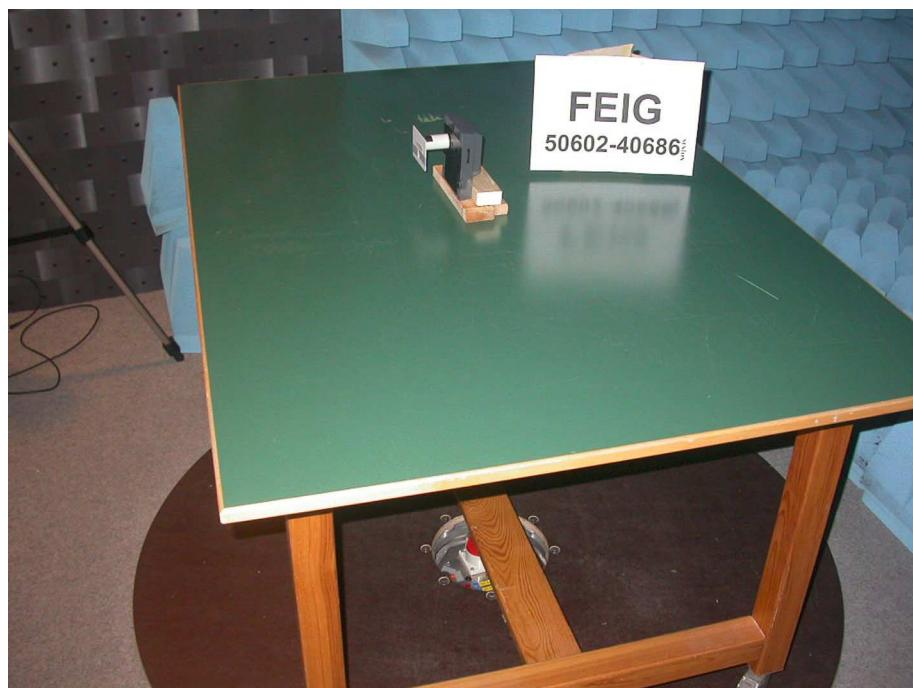
**Test setup for radiated emission test
