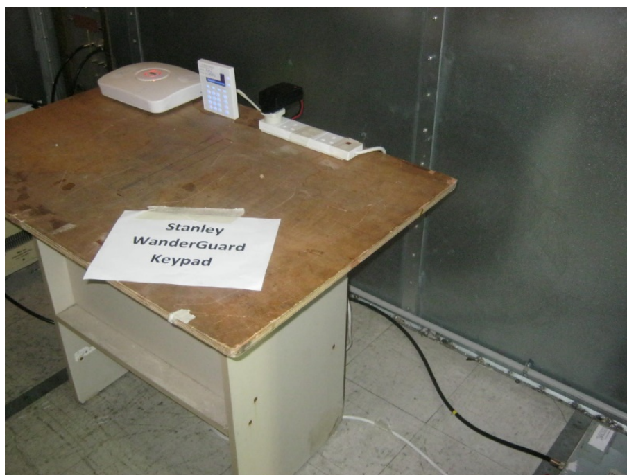
Figure 3. Conducted Emission from AC Mains (AC/DC adapter type 2) Test Setup
