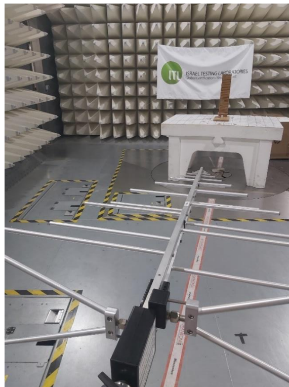
Figure 2. Radiated Emission Test, 30-1000MHz
