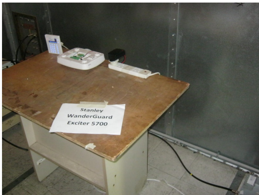
Figure 4. Conducted Emission from AC Mains (AC/DC adapter type 2) Test Setup
