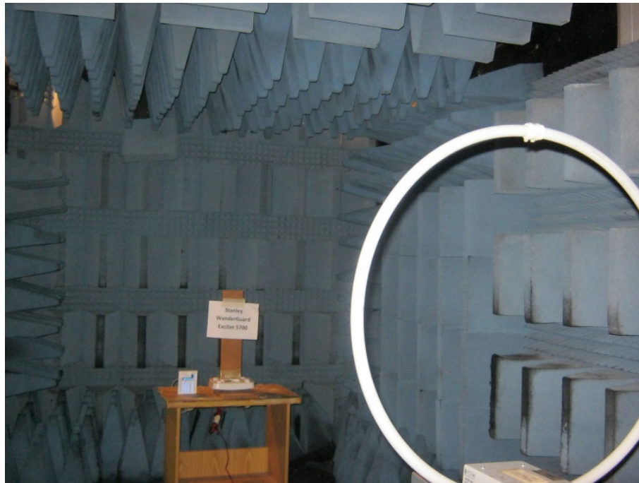
Figure 5. Radiated Emission Test Setup
