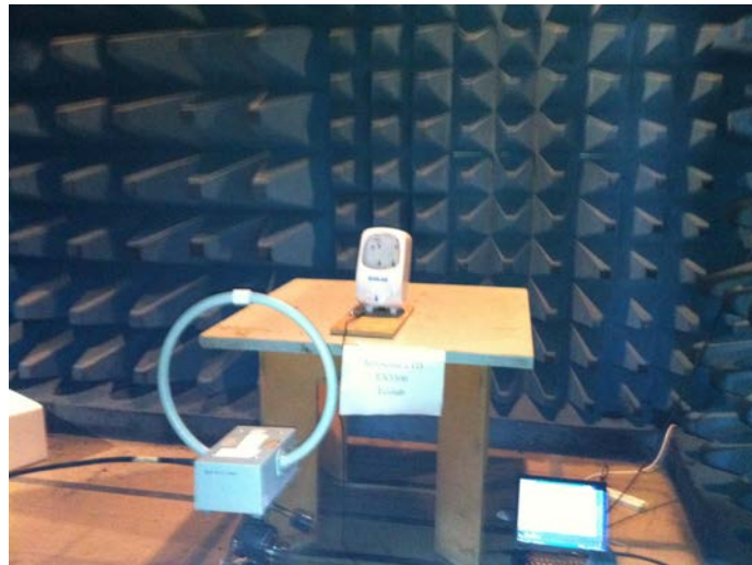
Figure 2. Exploratory Radiated Emission Test Host ECOLAB
