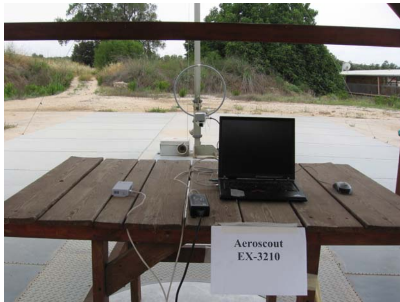
Figure 2. Radiated Emission Test
