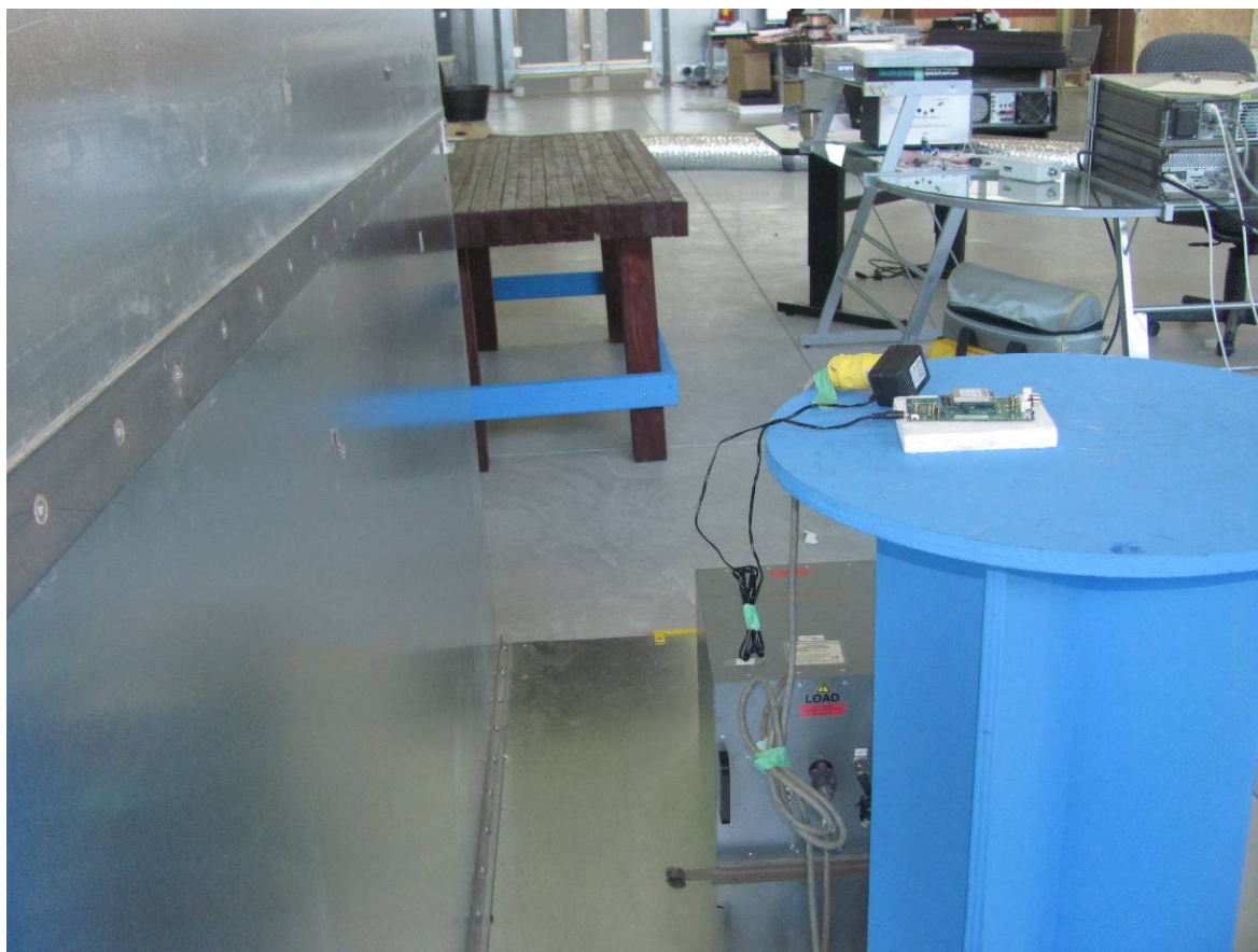
Figure 2: Power line conducted emission setup – photo 2
