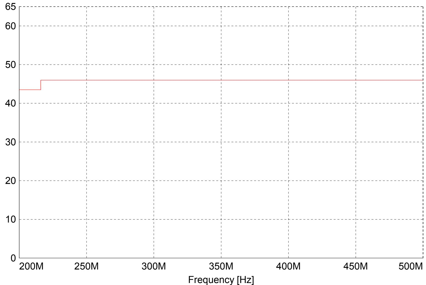
— LIM FCC Class B QP/AV      Voltage Amplitude FCC Class B
