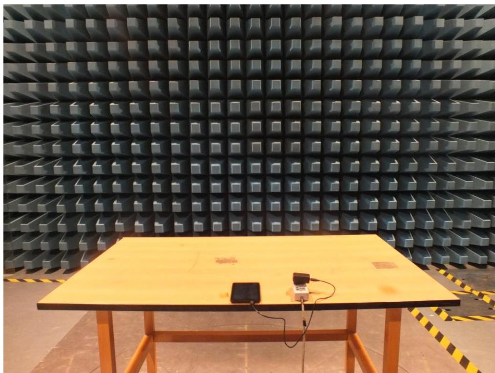
FCC Part15C Radiated Emission above 1GHz
