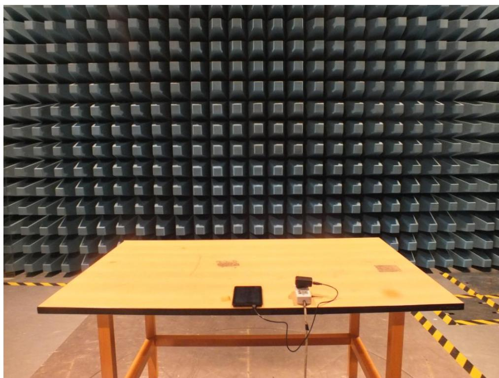
AC Conducted Emission Test Setup
