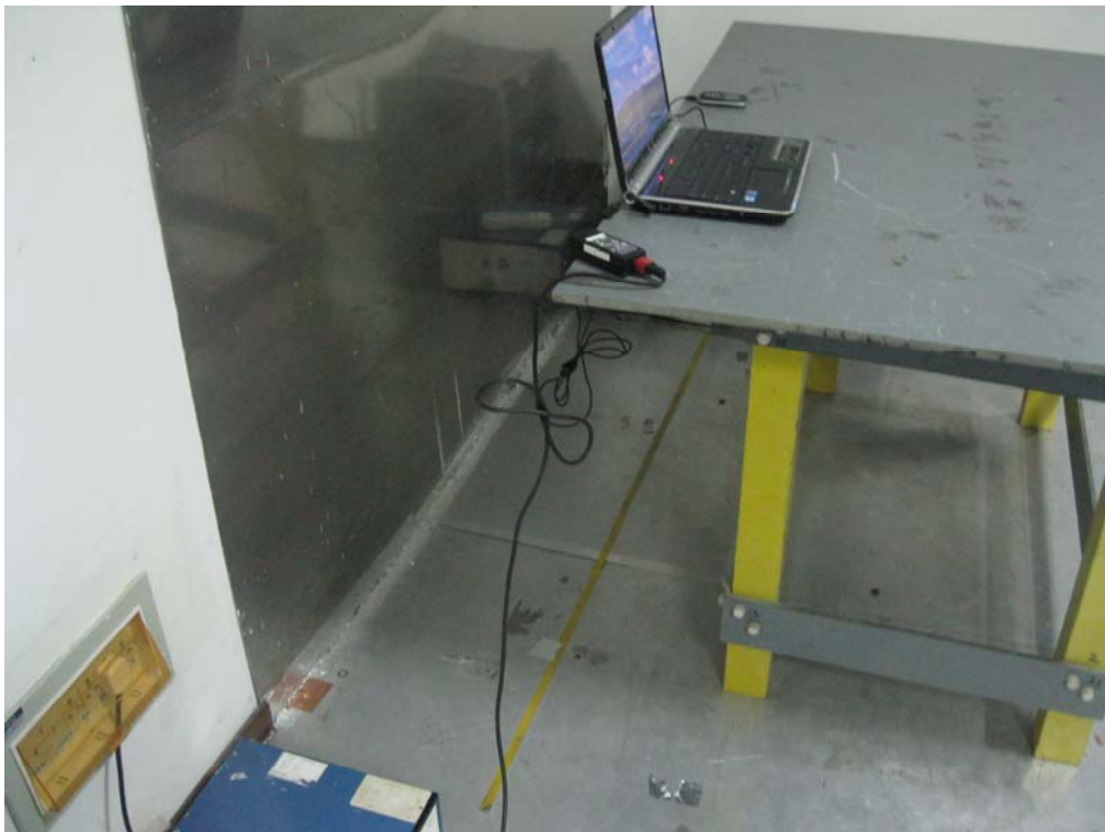
Conducted Emissions Test Setup - Side View
