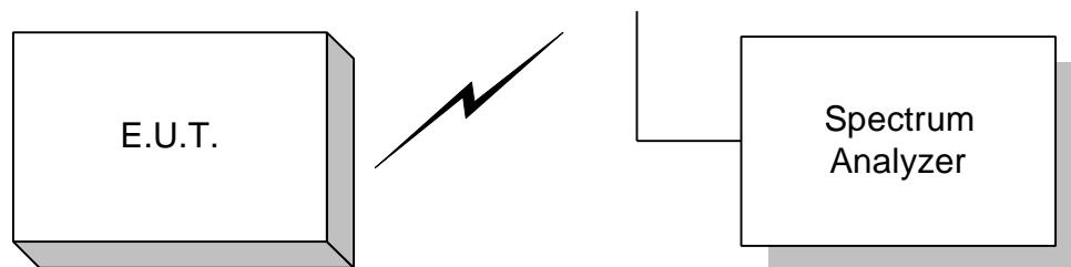
**Outdoor Test Site For Radiated Emissions**
