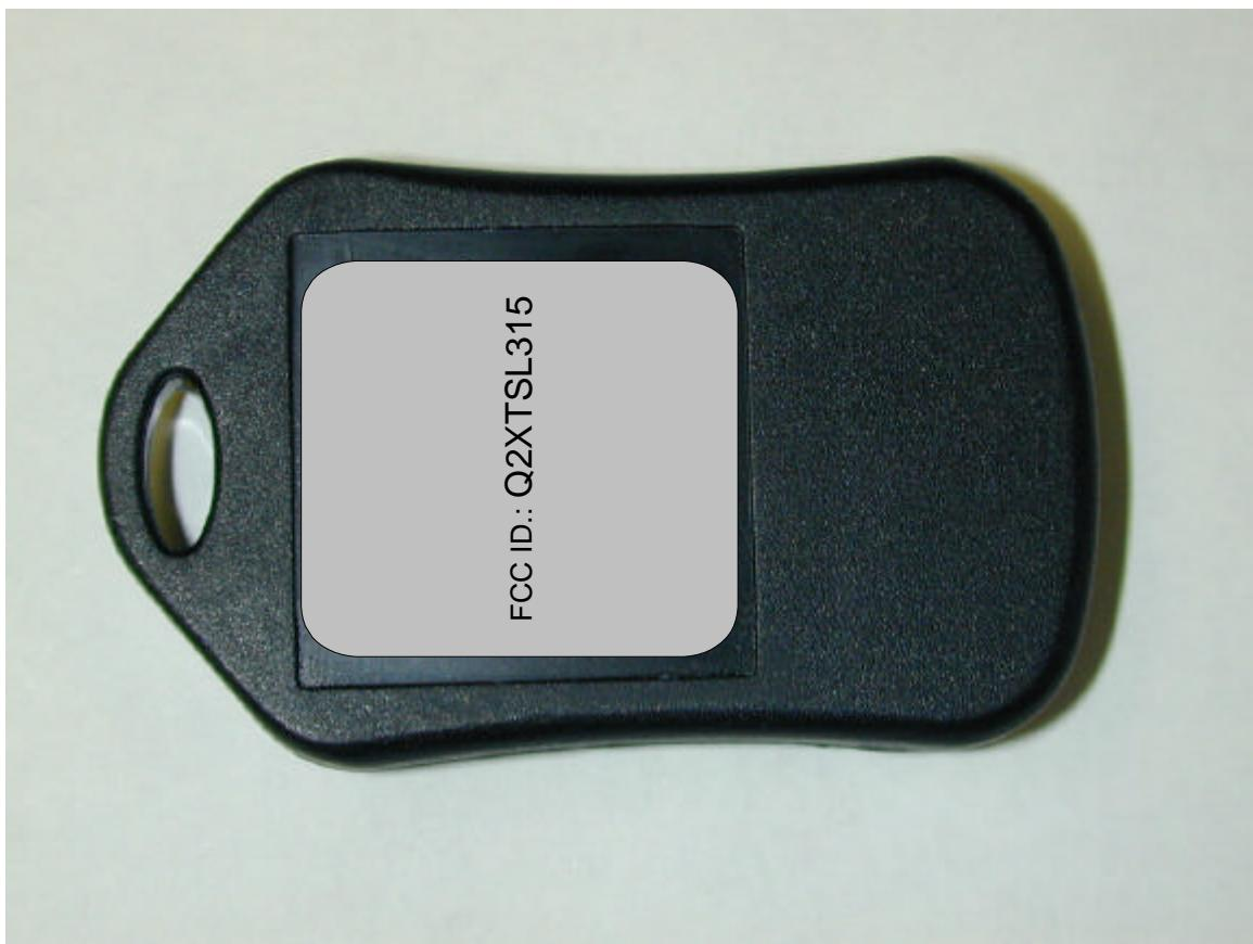
The label is printed with permanent ink on a durable decal material. The dimension of the label is 1" x 1".
