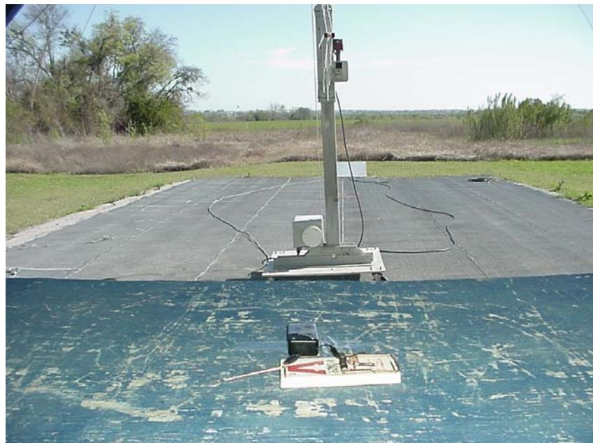
Radiated Emissions – EUT on its side
