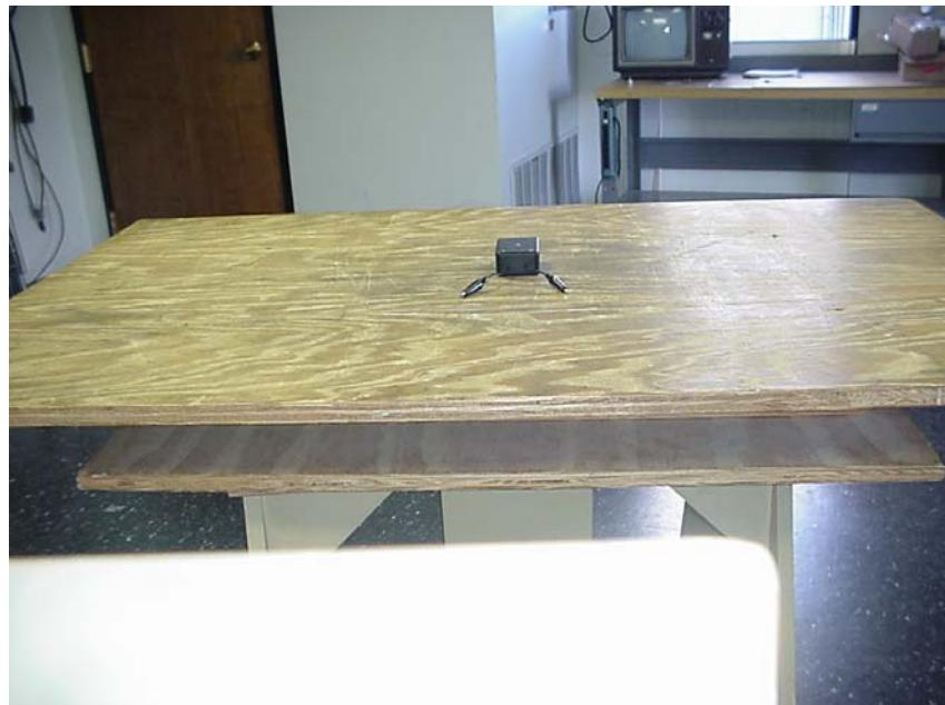
Microwave Radiated Emissions – rear view of EUT on its backside
