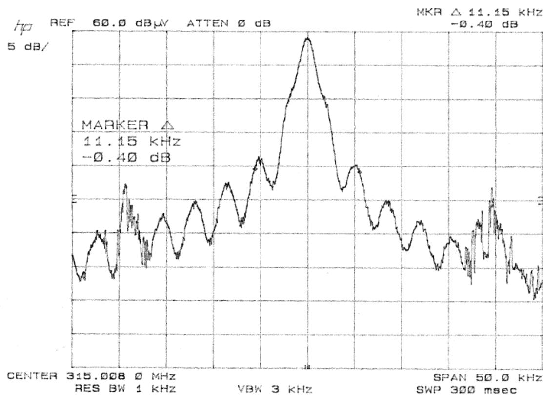
Note: The permitted bandwidth limit is 787.5 KHz. 25% of 315 MHz is allowed.
