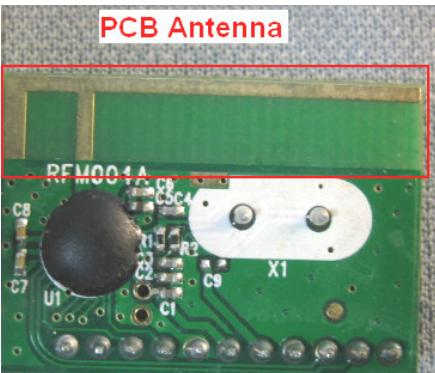
A photograph of a green printed circuit board (PCB) showing various electronic components. A red rectangular box highlights a specific area on the left side of the board. The text "PCB Antenna" is overlaid in red at the top left of the image. The highlighted area contains a black circular component, likely a chip antenna, and some surrounding circuitry and labels like "RFM001A", "C8", "C7", "U1", "C1", "C2", "C3", "R1", "R2", and "X1". |
