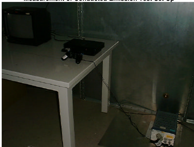
Measurement of Conducted Emission Test Set Up
