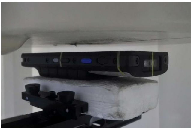
Front, Test Separation 10 mm for Battery2&3
