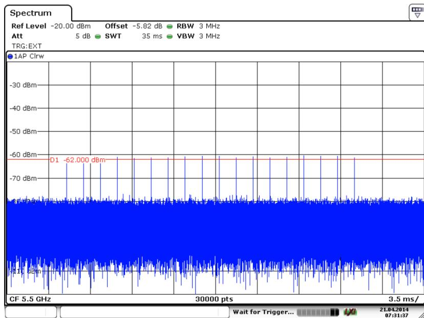
**<40MHz / 5510 MHz> Radar Type 1****Radar / DFS detection threshold level and the burst of pulses on the Channel frequency**
