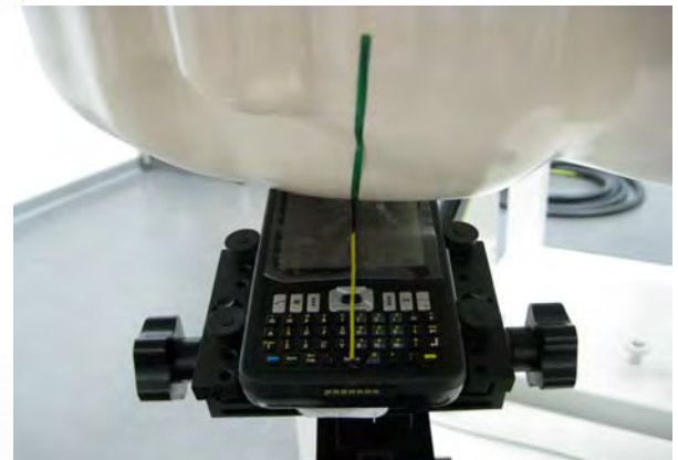
Fig.4 Right Head Section / Ear-Tilt Position(15°)
