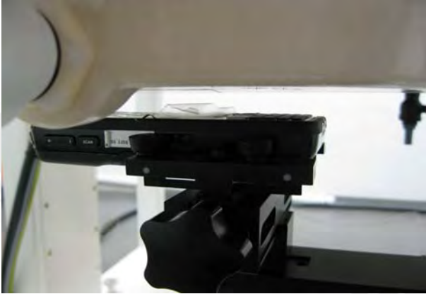
Fig.7 EUT front to flat phantom
