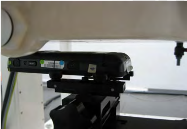
Fig.8 EUT back to flat phantom
