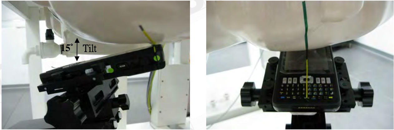
Fig.6 Left Head Section / Ear-Tilt Position(15°)
