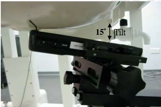
Fig.4 Right Head Section / Ear-Tilt Position(15°)
