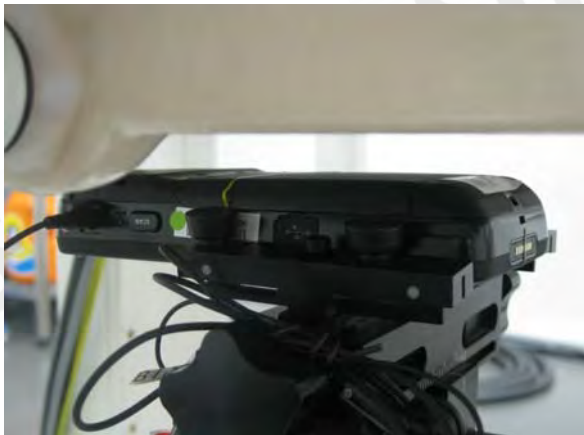
Fig.9 EUT back to flat phantom (With headset)
