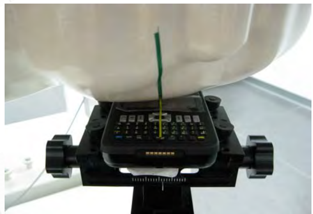
Fig.5 Left Head Section / Cheek-Touch Position
