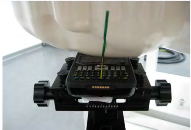
Fig.3 Right Head Section / Cheek-Touch Position
