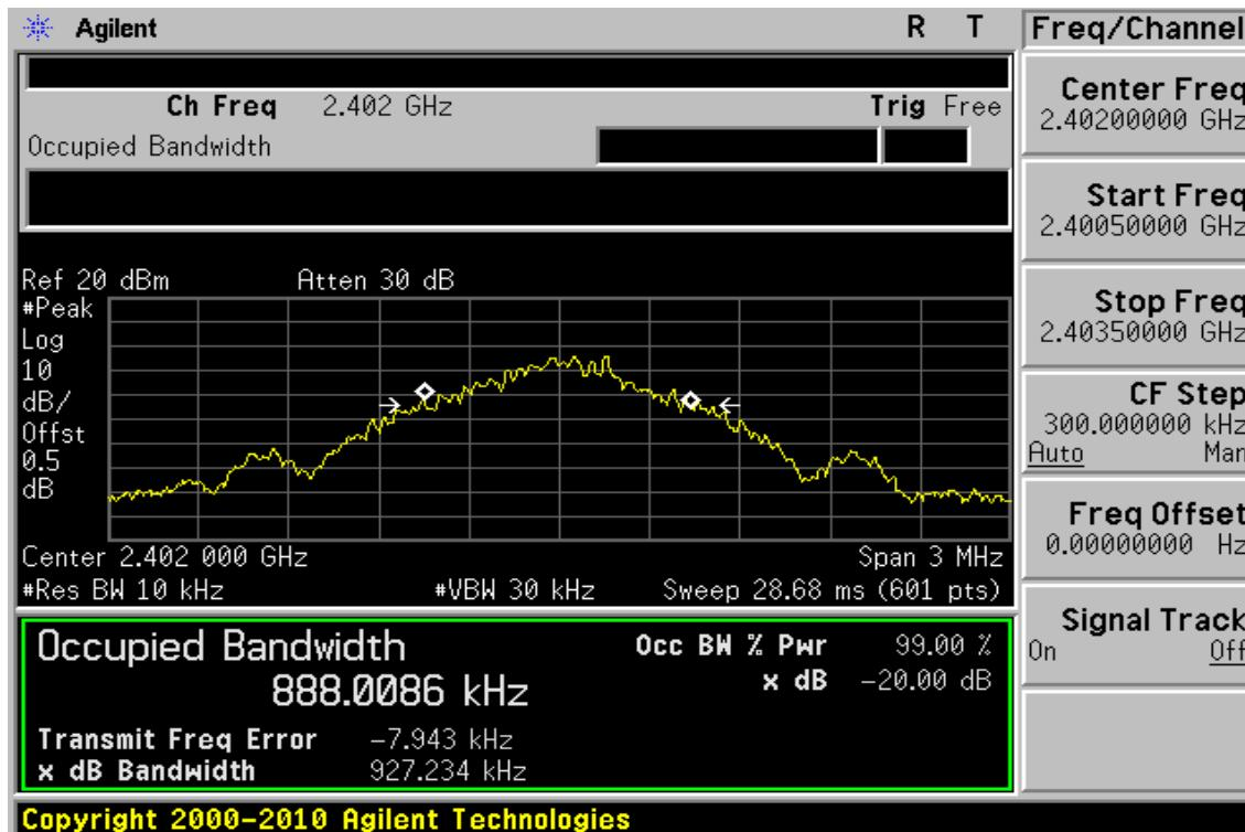
**20dB Band Width Test Data CH-Mid (BDR mode)**
