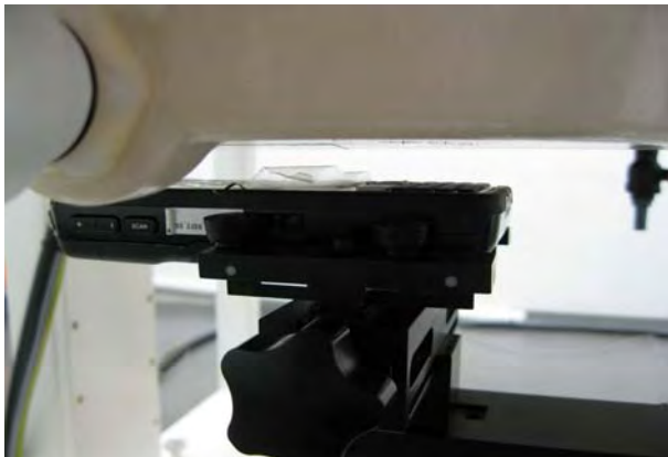
Fig.7 EUT front to flat phantom
