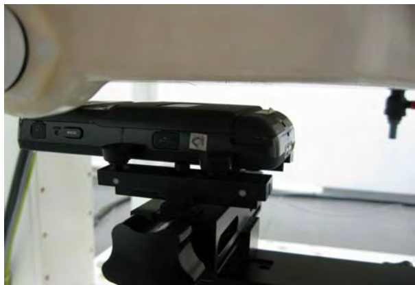
Fig.8 EUT back REID to flat phantom
